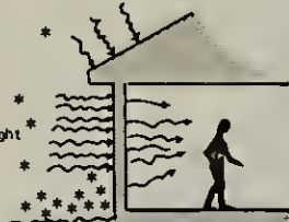
Gamma radiation can penetrate light materials. It loses some of its strength, however, when it passes through.
