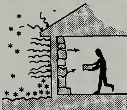
The thicker and heavier the material the more gamma rays are blocked out; therefore fewer pass through to cause injury.
